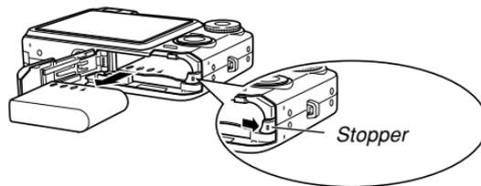
3. Release the stopper and pull the battery from the camera.
